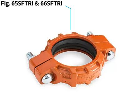
Figure 65SFTRI & 66SFTRI Standard Weight Flexible couplings are designed for use in piping systems where flexibility is desired. They allow for pipe movement caused by seismic action and thermal variations, and will also attenuate noise & vibration transmitted through the piping system.
